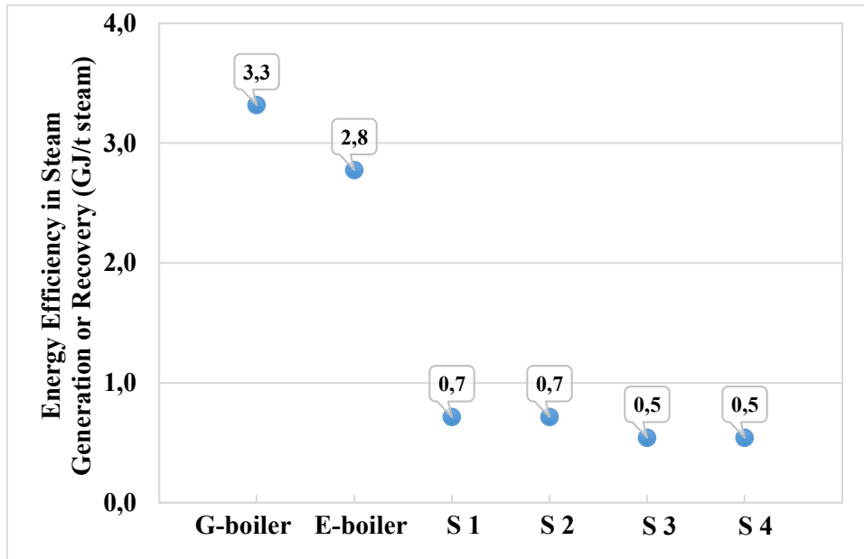
Figure 4. Energy efficiency of steam generation and recovery in Scenarios 1 to 4. (S 1-S 4: Scenario 1-Scenario 4)
